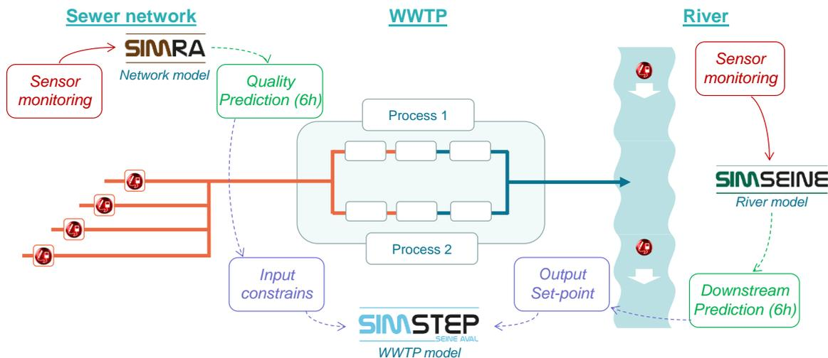
Figure 1. Diagram of an integrated management of the system made by the sewer network, the WWTP and the river. (Red color represents the monitoring, green color represents quality predictions and purple represents the constrains and output set-point)
