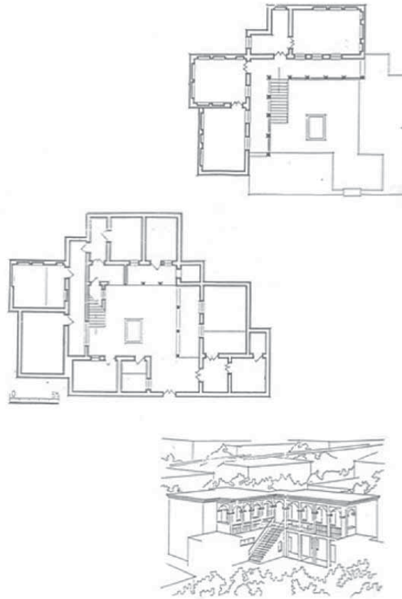
FIG. 13. Kashghar. Plans and drawing of a Uighur house. (Adapted from Rozi, 1995, p. 166.)
