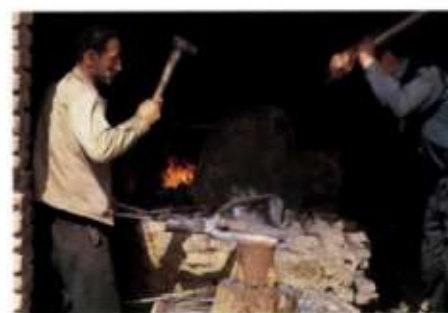
▲ A smithy in Iran today. Two metalsmiths are hammering the heated metal before shaping it.
